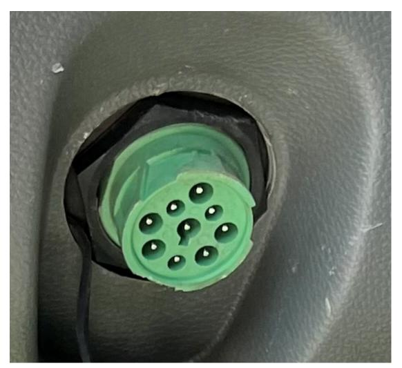
Figure 4. 9-pin OBD connector used for J1939
